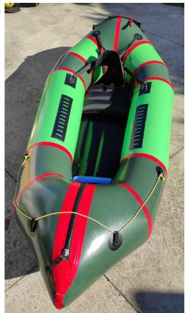
5. WW255 light blue. Full integrated floor/seat, new high strength thigh brace back rest attachment, new curved floor. Bow TiZip. **CURRENT MODEL**
