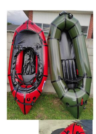
4. WW255 two tone green, red seams, with TiZip in bow. Integral floor seat with extra seat. Thigh braces included. This has the latest curved stern shape. Prototype with the integral floor, but this one was not as thick, hence the booster seat.
